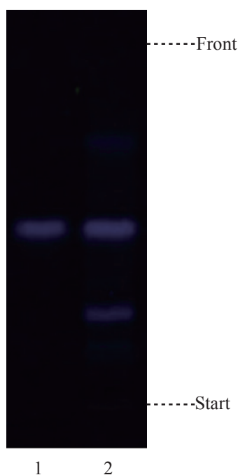
Figure 5 A reference TLC chromatogram of Wikstroemiae Radix extract observed under UV light (366 nm)
