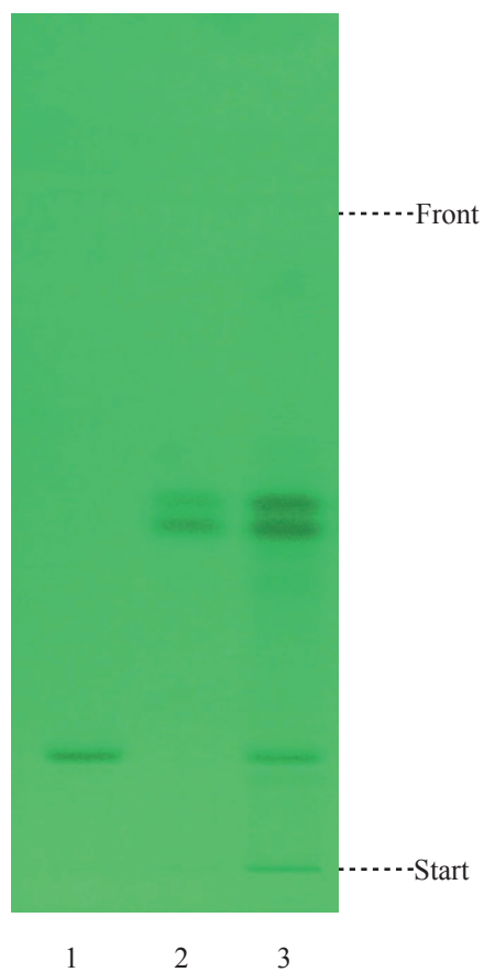
Figure 3 A reference HPTLC chromatogram of Garcinia Resina (unprocessed) extract observed under UV light (254 nm)
