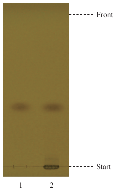
Figure 5 A reference HPTLC chromatogram of Cynanchi Paniculati Radix et Rhizoma extract observed under visible light after staining
